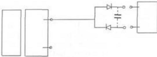
no diodes in XIX century. Still the "Avramenko plug" is a component of the known voltage-doubling circuit or monophasic input of any bridge rectifier (Fig. 6).
