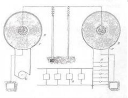
**Fig. 3. Electric circuit of N. Tesla's device for resonance system of electric power transmission [9].**
